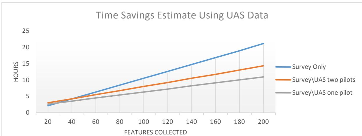
Figure 3: Chart Depicting Growth in Time Savings using UAS
